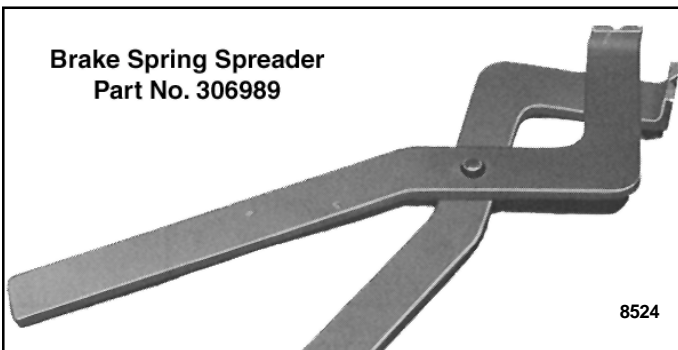
Figure 7-4. Special Tool for Removing Brake Spring.
