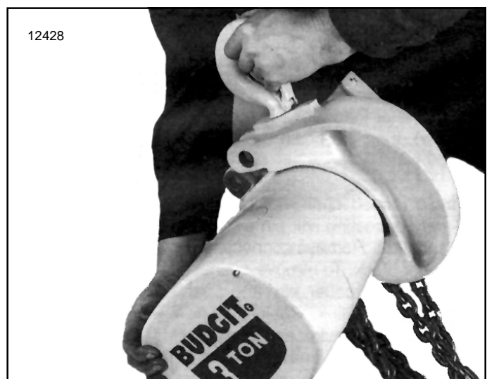
Figure 7-2. Removing 3 Ton Hanger Bracket from Hoist Frame
