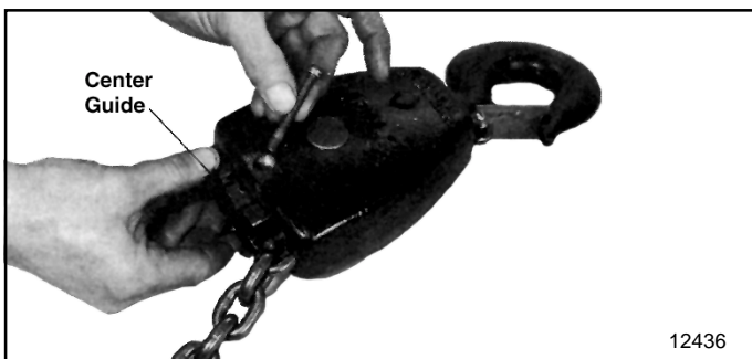
Figure 7-24. Removing Chain Center Guide from Double and Triple Reeved Lower Block Assembly
