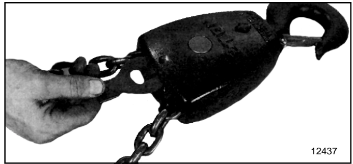
Figure 7-25. Removing Sprocket Pin Lock on Double and Triple Reeved Lower Block Assembly.
