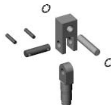
Figure 11. 3 Ton (3000 kg) Hoist to Trolley Assembly
