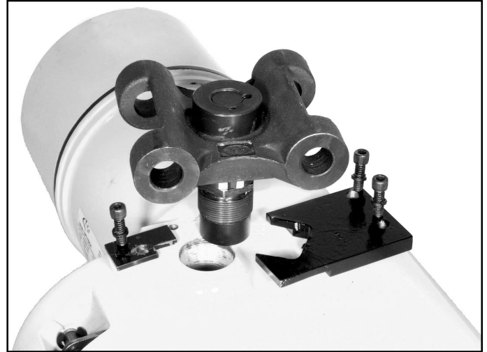
Figure 7-20. Removing Suspension Lug (1/4 through 1 Ton Models)
