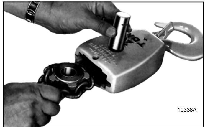
Figure 7-29. Removing Coil Chain and Sprocket on 2 through 5 Ton Lower Block Assembly (Link Chain Model)
