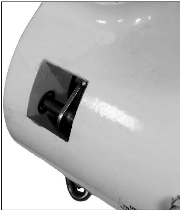
Figure 7-13. Removing Chain Guide Support Pins
