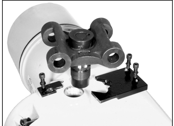
Figure 7-20. Removing Suspension Lug (1/4 through 1 Ton Models)
