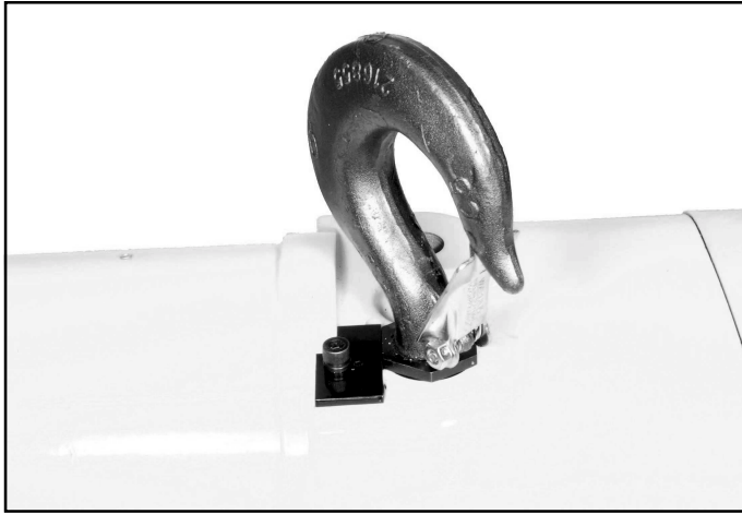
Figure 7-18. Removing Upper Hook and Hook Nut from Hoist Frame (1/4 through 1 Ton Models)
