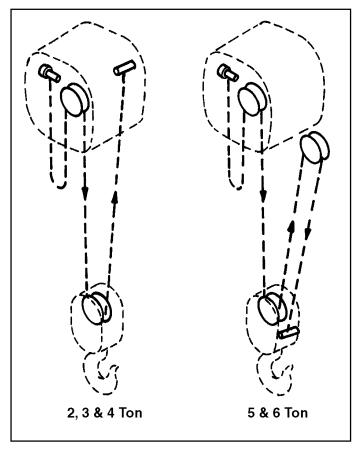
Figure 7-9. Reeving for 2 thru 6 Ton Models
