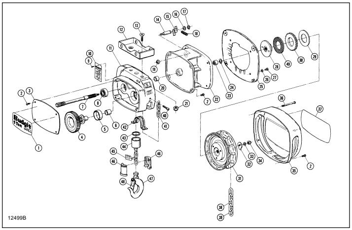
Figure 9-2a. 1 Ton Trolley Hoist Models
