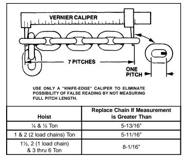
Figure 5-2. Checking Coil Chain Using Vernier Caliper
