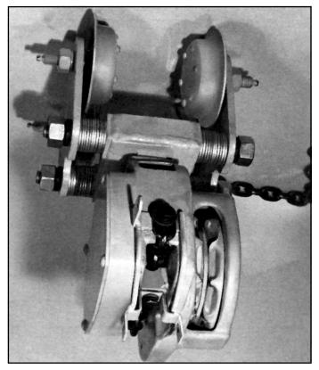
Figure 10-1. Chain Container Bracket
