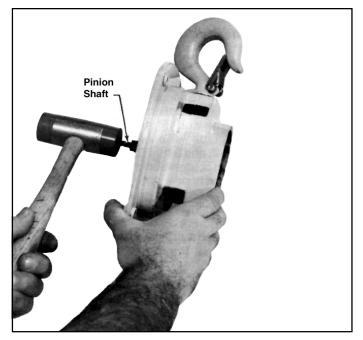
Figure 7-3. Removing Pinion Shaft
