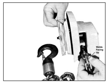
Figure 7-8. Installing Load Chain
