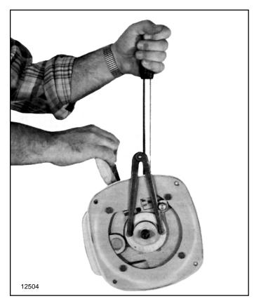
Figure 7-2. Removing Load Brake Flange
