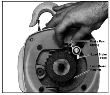
Figure 7-5. Installing Load Brake Pawl
