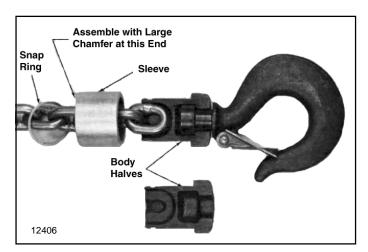
Figure 7-1. Lower Hook Connection
