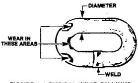
FIGURE 4-4. TYPICAL WEAR ON LINKS
