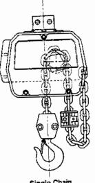
Single Chain 1 & 2 Ton Hoist CAUTION: Top Suspension must be centered over bottom hook. See Fig. 5-3 Top Suspension orientation.
