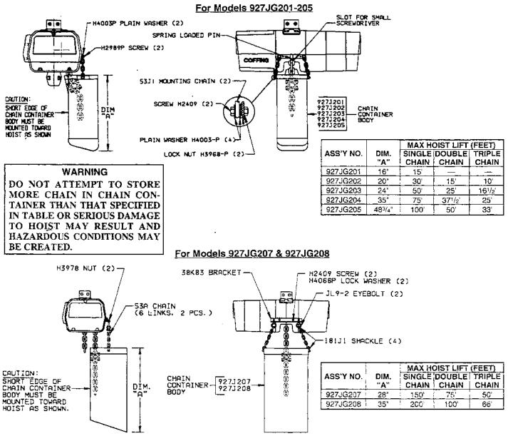
FIGURE 2-2. CHAIN CONTAINER INSTALLATION
