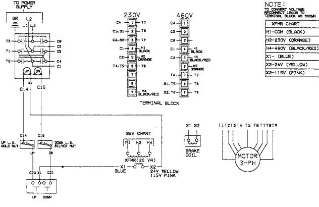
FIGURE 7-1. WIRING DIAGRAM 230/460V, 3 Phase, Single Speed Hoist
