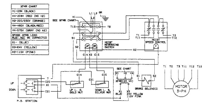
• INDICATES SPLICE CONNECTIONS; CONNECT IDENTICAL TERMINALS TOGETHER
