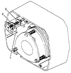
FIGURE 5-1. LIMIT SWITCH ADJUSTMENT
