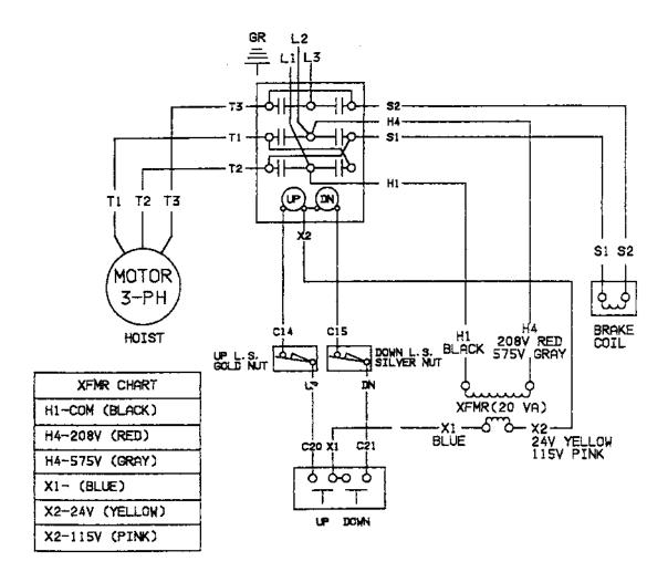
FIGURE 7-2. WIRING DIAGRAM 208V or 575V, 3 Phase, Single Speed Hoist
