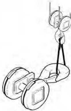
Figure 3-12 Lifting Bottom Block
