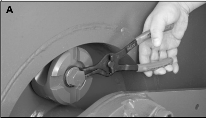
Figure 8 – Reversing the Cable Anchor
