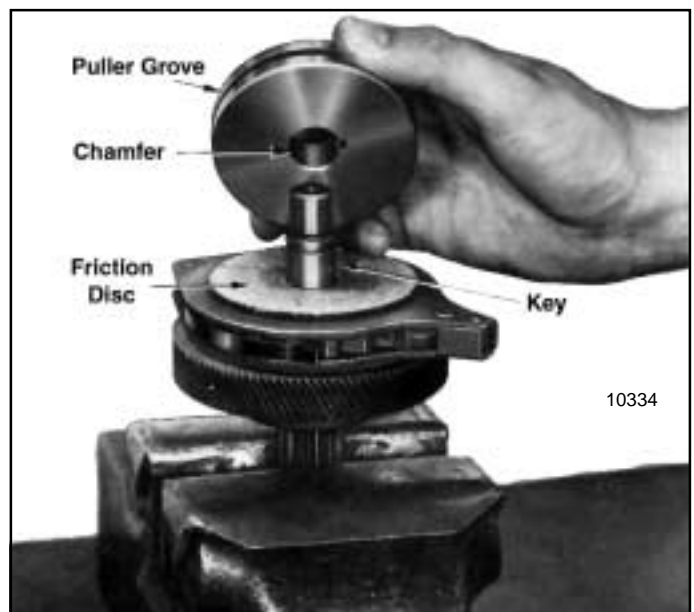
Figure 7-22. View Showing Load Brake Flange Removed
