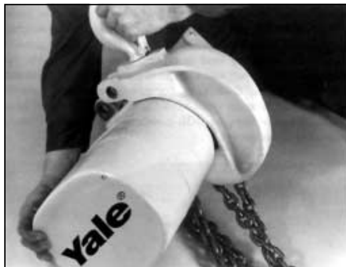
Figure 7-3. Removing 3 Ton Hanger Bracket from Hoist Frame
