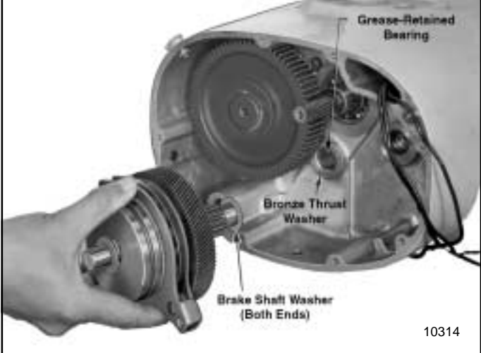
Figure 7-7. Removing Load Brake and Clutch Assembly (1/4 & 1/2 Ton Hoists)
