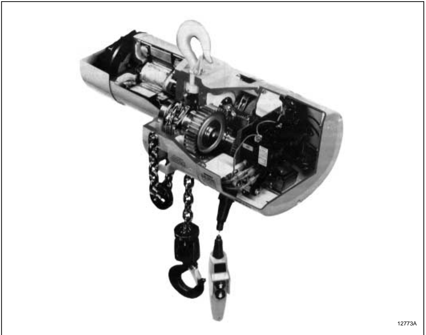
Figure 1-1. Cutaway View Of Typical Yale Electric Hoist
